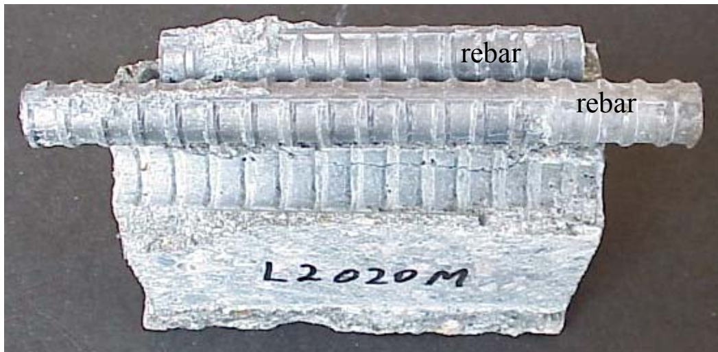
Figure 12 – No corrosion is seen on the low density concrete sample surface treated with MCI 2020M inhibitor.
