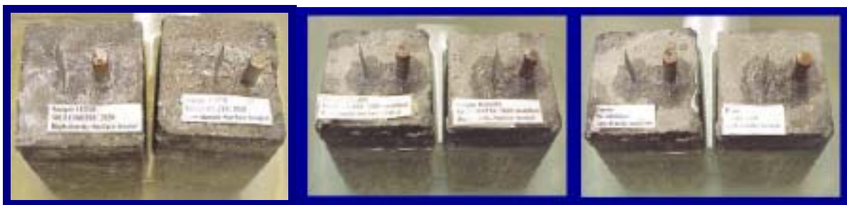
Figure 1 – The concrete samples partially immersed in a 3.5% NaCl solution.
