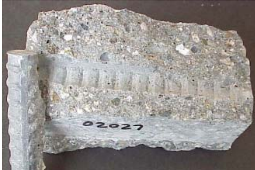
Figure 11 – No corrosion is seen on the low density concrete sample surface treated with MCI 2020 inhibitor.
